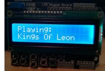
This one is for the Spotify people. We've created a small project that makes use of the Arduino and LCD Keypad shield to create a Spotify remote control. This will show the current playing song as well as adding Play/Pause, Prev and Next functionality to it.
